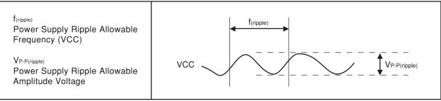
Figure 21.1 Timing of Voltage Fluctuation
